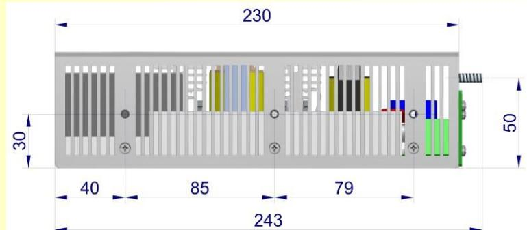
Lateral fixing holes 6 x M4 (screw torque < 1.6 Nm). Maximum screw deep 6 mm.
