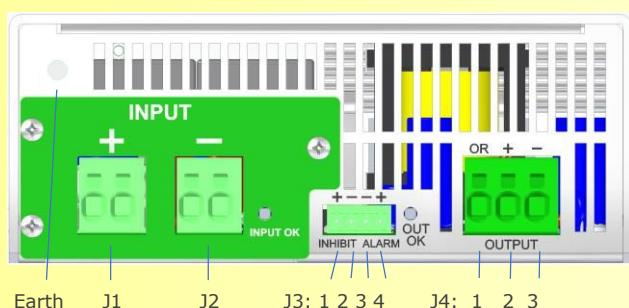
Note 1: maximum spring terminals cross section cable 6mm<sup>2</sup> or 10 mm<sup>2</sup> for solid
